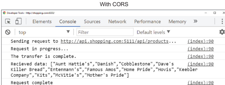
Figure 18.14 With CORS enabled, cross-origin requests can be made and the browser will make the response available to the JavaScript. Compare this to figure 18.12, in which the request was blocked.
